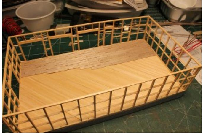
It required hours to build 26 roof trusses, each with 16 individual cut pieces and 14 NBW castings. The end trusses were modified slightly to accept the exterior siding at the gables.
