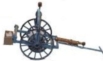
Fig 2. First is the basic frame. It should be about 11.50 feet long and 3.50 feet wide. The pole can be either round, square or something in between, depending on the original maker and what repairs were done to keep the cart in service. Wood and sometimes steel would be the material of choice. Remember, weight would have been a major consideration.
