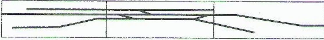
Measuring just 15 inches by 144 inches, our HO scale portable switching layout has less than half the area of a standard 4' x 9' sheet of plywood, yet is designed to offer challenging and prototypical operation. The six switches create a small yard featuring a run-around track and four spurs, which serve a total of nearly a dozen different industries.
