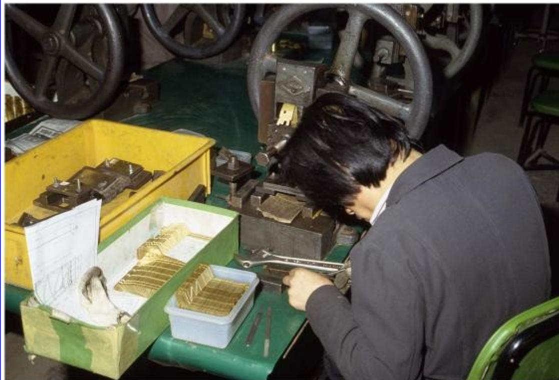
**This man is making final preparations to punch holes into the ends of 600 HO scale outside braced open hopper car sides. Each of the steel dies in the yellow tub were created to punch a single hole or series of holes into brass car sides that will be fed one at a time into the rotary punch. You can see a caboose side hanging out of the opening in the punch closest to us. That particular photo etched sheet was fed into the punch, the wheel rotated to actuate the punch, and the window openings**
