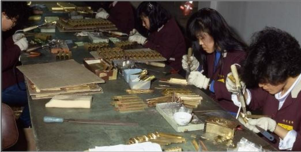
**The first two workers in this assembly line are using soldering jigs to assemble the sides, back wall, and roof of an HO scale steam locomotive cab. From there the subassemblies are passed down the line and each worker adds another part to complete each cab.**
