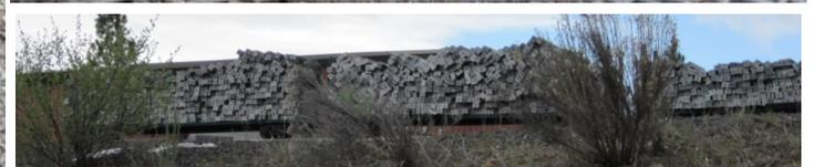
Above right: **Flat cars of ties ready to be laid.** Below left: **Aluminum rail and wood ties are being replaced with plastic ties and steel rail (no steel rail shown here).** Below right: **Stacks of track panels in the yard.**
