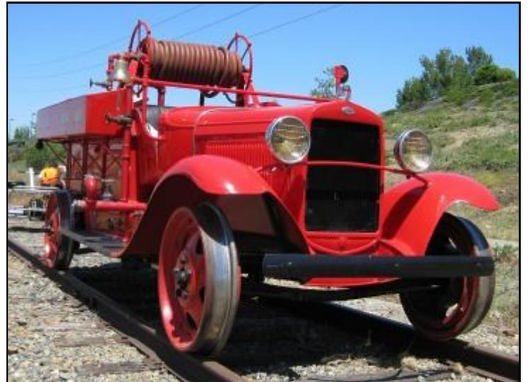
The California State Railroad Museum had this 1931 Ford Model AA Fire Truck on display. This 4 cylinder, 40 hp fire truck was operated by the San Diego & Eastern Railway as MW 1003. It had the ability to refill it's tanks at trackside water tanks and was in service for almost 50 years.
