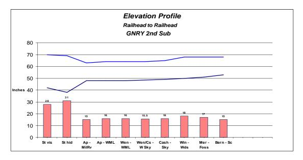
The bars show the deltas in inches between the upper and lower levels at various points along the layout. The lines above represent the lower and upper levels showing both elevation and differences between the levels.
