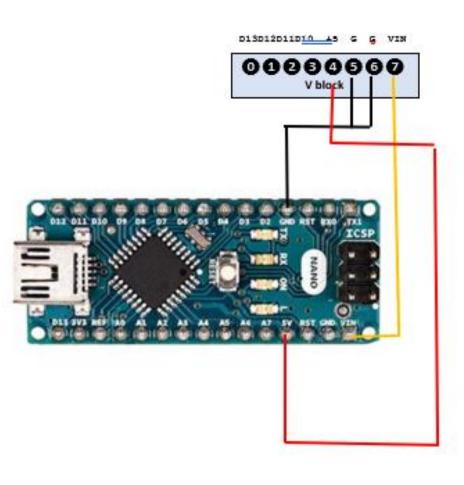
Black – Ground Red - +5 volts Green – sensor inputs Yellow – VIN Blue – output to alert
