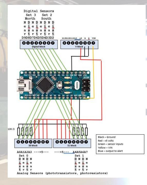
Add the digital output lines to the output/power block
