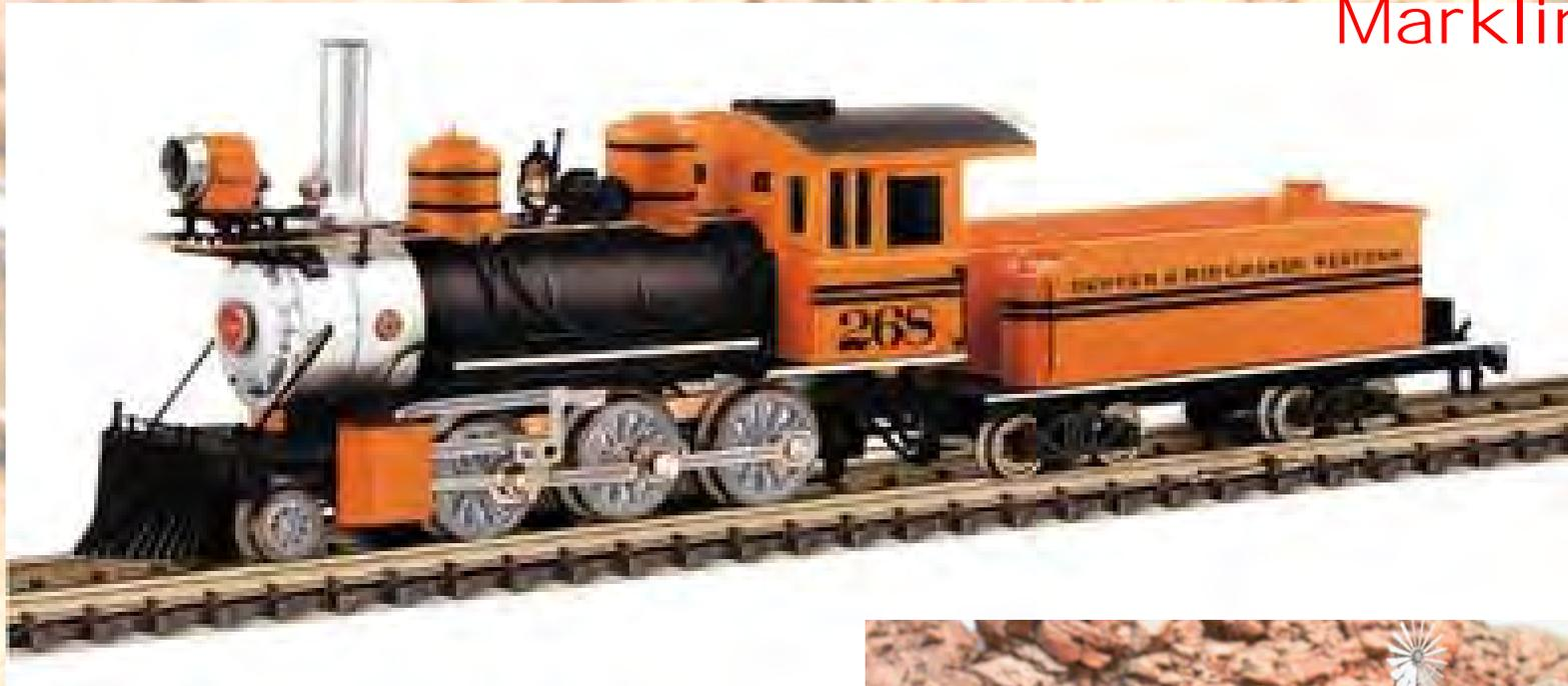
**Brass superstructure on Marklin chassis; marketed as part of Marklin's Mini-Club Z-scale line, but model scales out to N-narrow gauge; the original #268 was a 2-8-0. (Re-painted and fitted with MT couplers at right.)**
