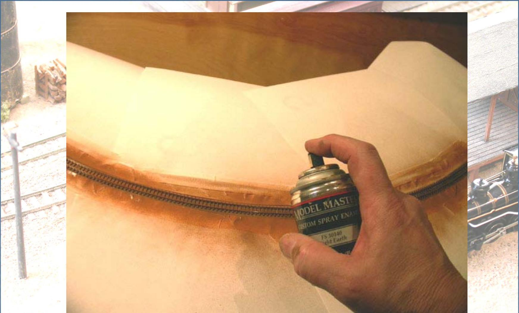
Mask adjacent terrain and spray both rail and ties with Testor's Master Modelers Light Earth or Floquil Rail Brown
