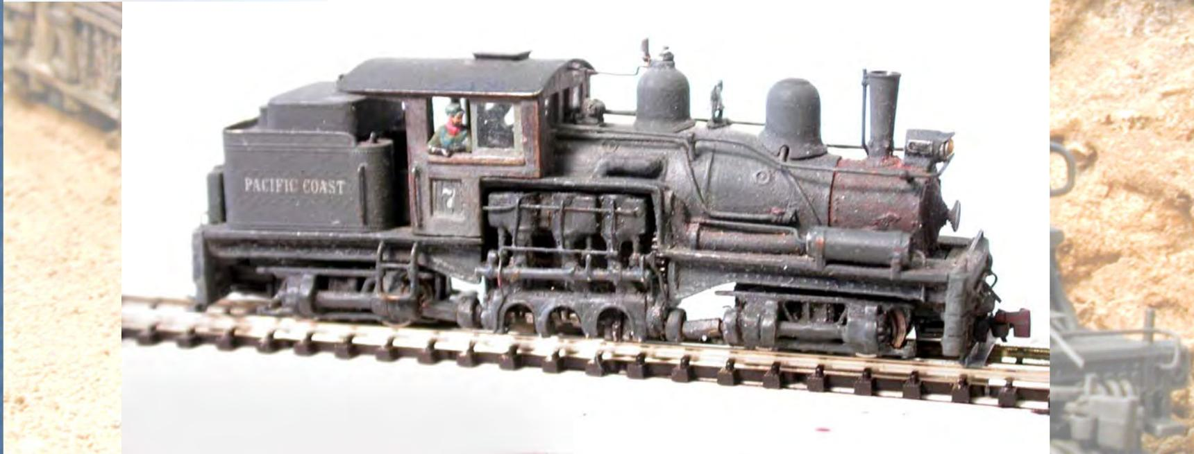
TWO TRUCK SHAY WITH OPERATING CRANK- AND DRIVE-SHAFTS SCRATCH-BUILT BY AUTHOR DURING 1980'S, TO RUN ON .256" (6.50 MM) GAUGE TRACK
