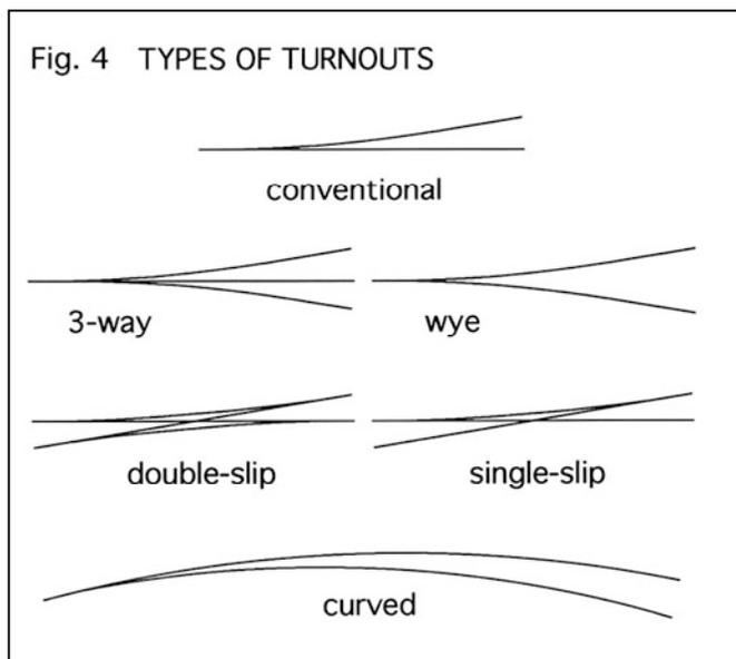
number) can better utilize limited space and may be acceptable for operation of shorter engines and shorter cars. Operating problems can be avoided by carefully designing the layout before laying any track.
