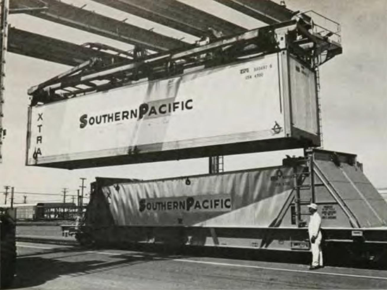
PIGGYBACK COFC: Southern Pacific is testing a flat car that will carry two stacked 40-foot containers. Built by ACF, No. 513300 is 18½ feet high over the load.
