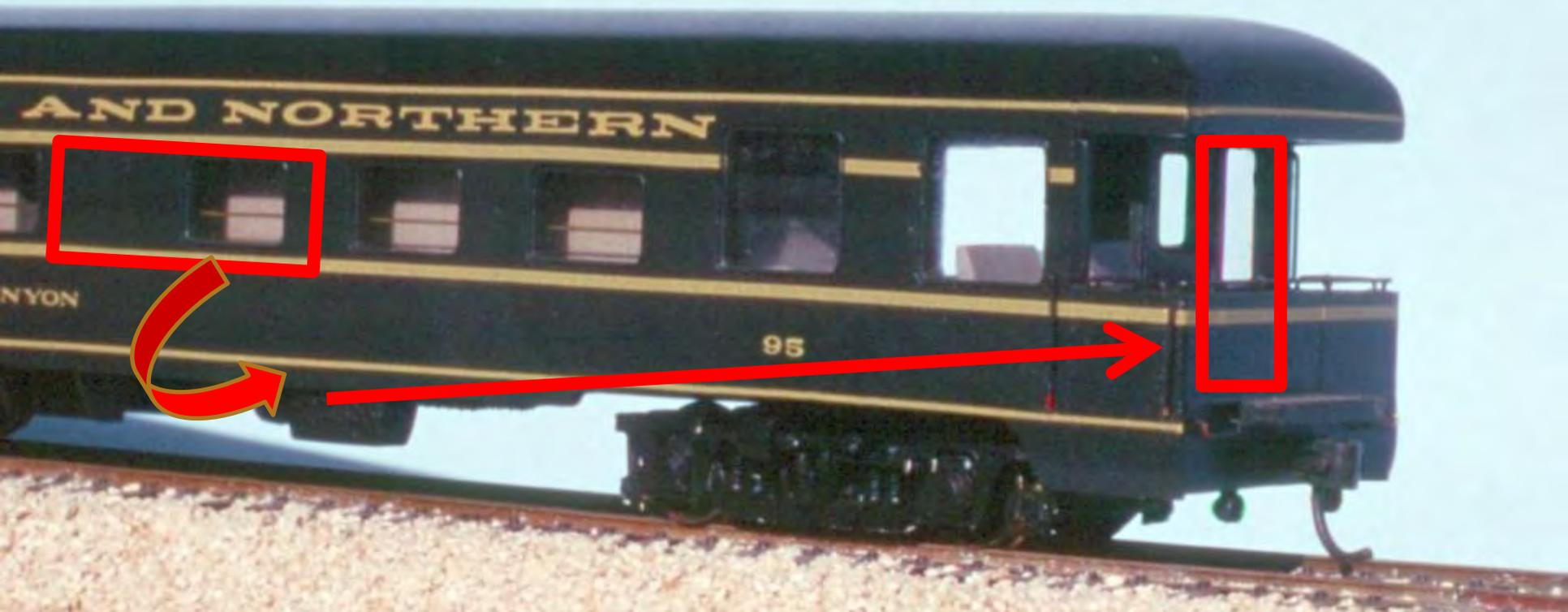
**End windows built from rotating side windows with long wall to provide tall windows, door made from small window and wall rotated 90 degrees, and filed thin to provide recess.**
