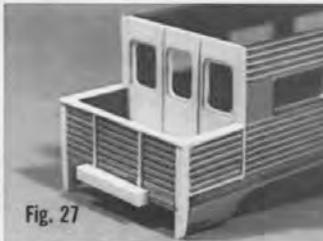
^ This car end was built using material from a wrecked car. Strips of styrene were used for dividers, corners, and striker. † File corner posts to match the side skirting after the cement has dried. Install
