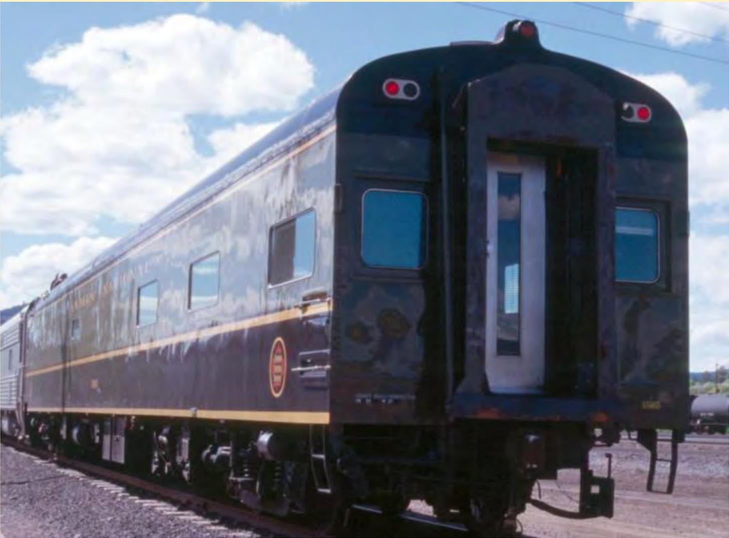
**CN “TAWAW” served as the diner on this BNSF Business train at Whitefish, Montana. The other cars were HEP equipped. This car was steam-heat equipped with motor-generator, so was coupled last, following the power car-sleeper.**
