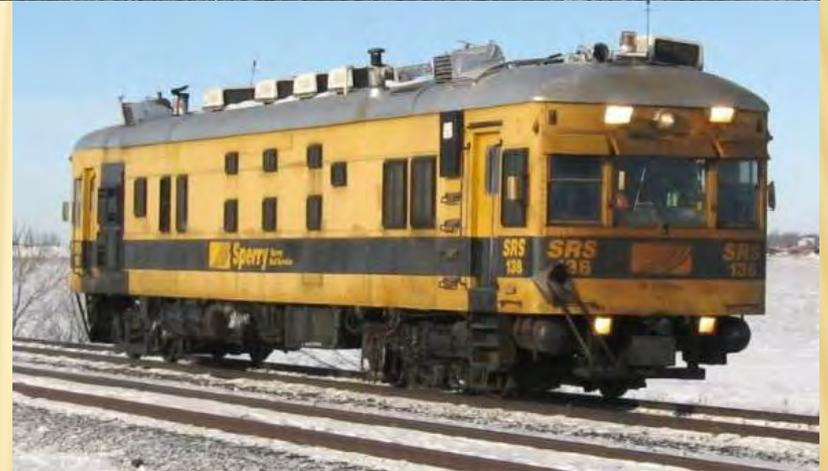
**Sperry Rail Service has provided rail inspection services on contract to the railroads since 1928. The process detects flaws in rails, then mark the spot and reports to the railroad.**
