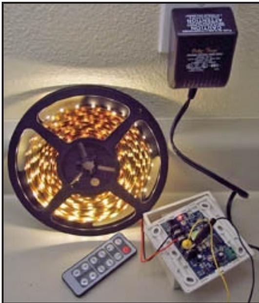
All the components parts are shown, the 12 vdc power supply, the dimmer control box, the dimmer remote, and the 5 meter reel of LED ribbon lights.
