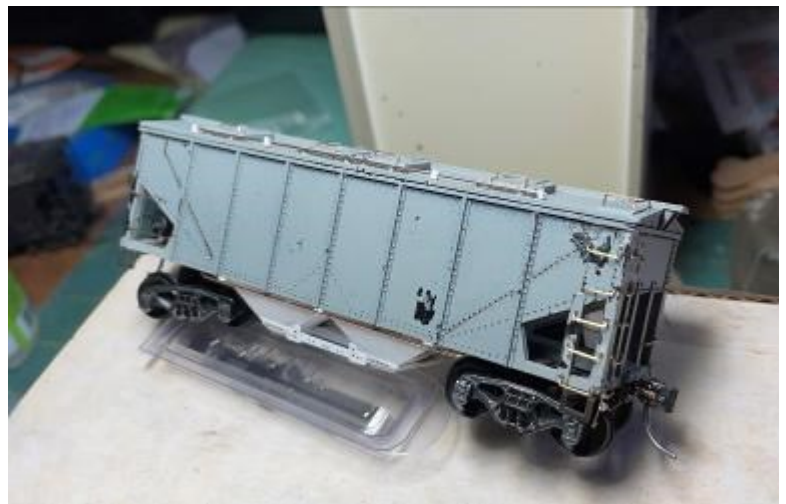
A second shot of the Varney rebuild. Here we can see the new outer slope sheet rivet lines made with Archer Fine Transfer rivets. Cement needed steeper slope sheets in order to be self-cleaning during unloading. Railroads didn't remove the old outer slope sheets – they just riveted in new ones at the correct 50-degree angle inside the car!
