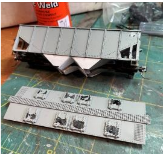
One of the two 55-ton rebuilt coal hoppers, in this case the Varney car, with oversized details removed and work proceeding to create the new hopper bays. Note how the slope of the new styrene overlays does not match that of the rivet lines on the bottom of the outer slope sheets.
