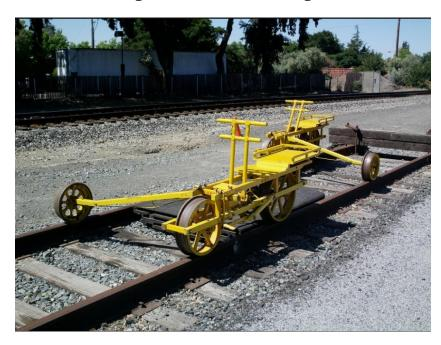
The car herewith illustrated facilitates a close inspection of a railroad, and it is claimed that by no other device can this be done so effectually. It is propelled by one person and has a device for carrying a second, thereby enabling a road master or inspector, when convenient, to avail himself of the services of a spare section hand or other man for the purpose of propelling him over the line, he being free to note all defects in alignment or surfacing.
